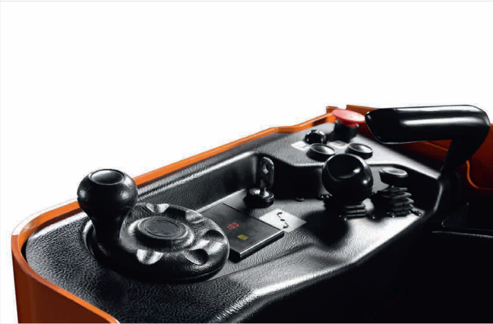
Easy driving with small electronic steering wheel
