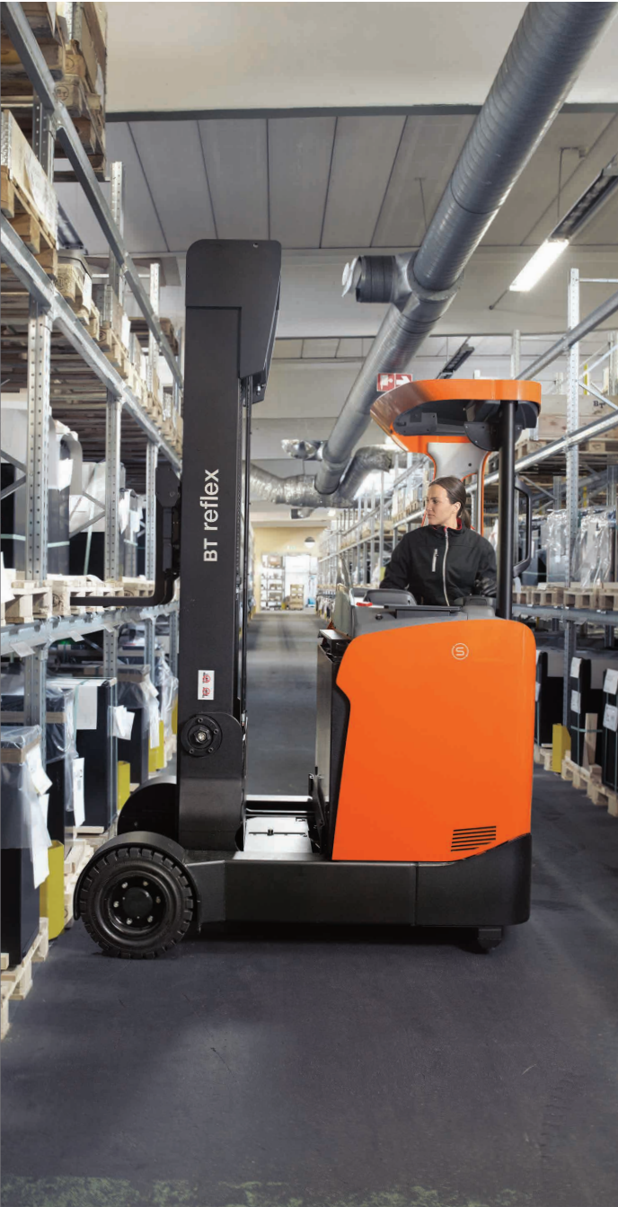
Superelastic tyres on all wheels and 145 mm ground clearance mean the BT Reflex O-series can handle outdoor surfaces, including gradients and transitions.
