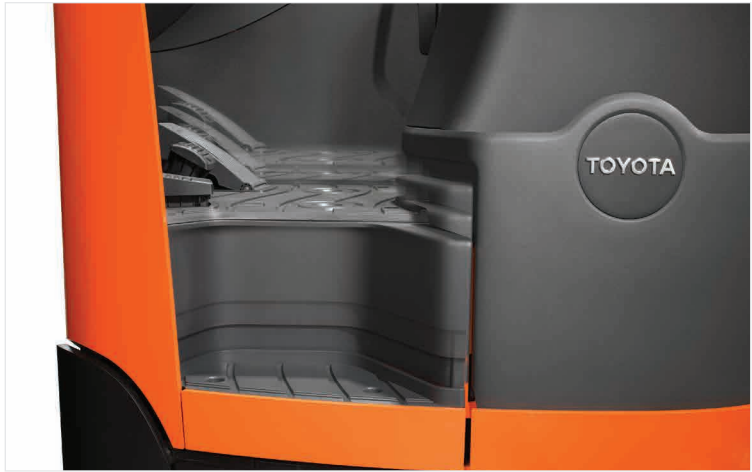
The driver compartment is adjustable to suit different driver sizes. The floor height can be adapted manually or electronically.
