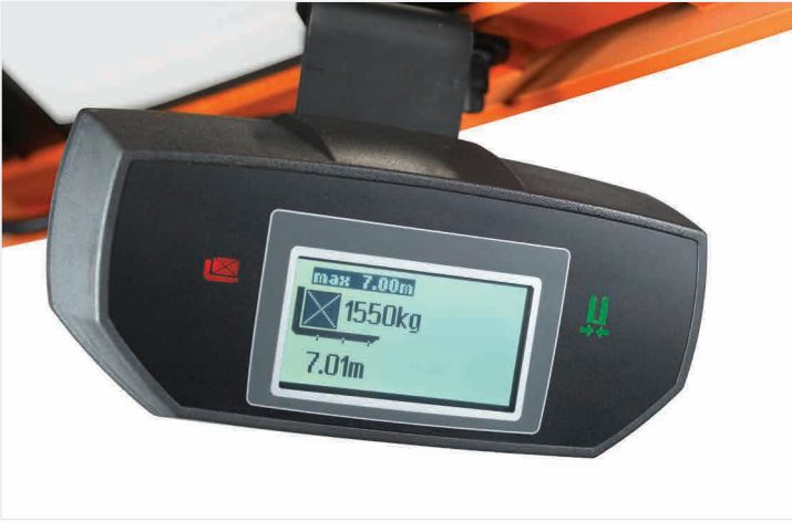
The overload warning system will warn the operator when the maximum lift height is reached for the load on the forks.
