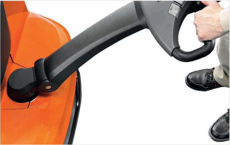
The tiller arm length is optimised for safety, keeping the operator's feet away from the truck
