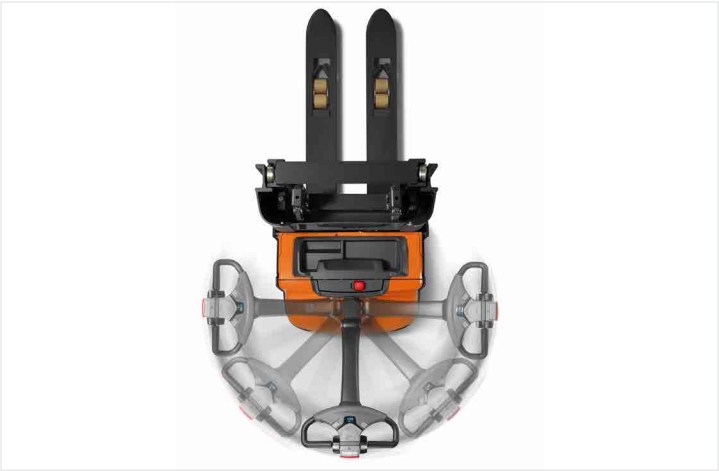
Automatic speed reduction when cornering as option for safe operations
