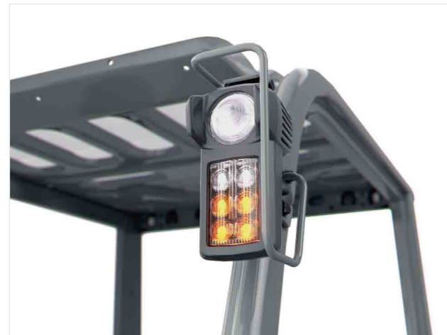
New front LED light for more visibility and improved productivity.
