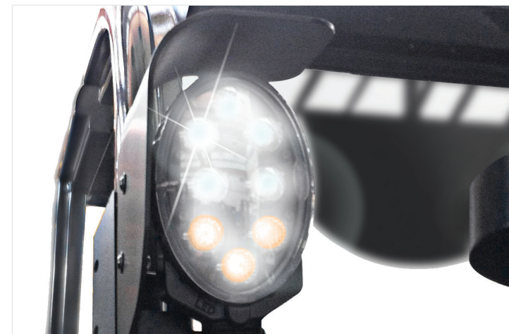
Powerful yet energy-efficient LED working lights increase visibility and allow work to continue in dark or unlit areas.
